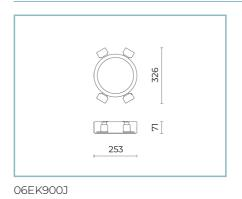
EKLEIPSIS SMALL recessed kit for plasterboard ceilings
