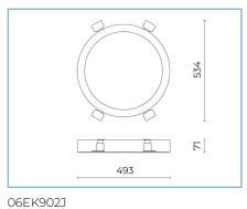
EKLEIPSIS LARGE recessed kit for plasterboard ceilings
