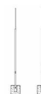
Palo rastremato base Ø 127 mm, testa palo Ø 102 mm + codolo Ø 60 mm H 90, codolo Ø 60 mm H 120 mm
